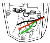
Strip the service wires going to the terminal block on the top entry bracket 3/4" (18 mm). Ferrules are recommended.
