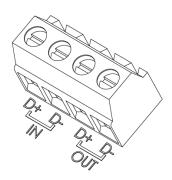
Form a daisy-chained network by connecting the cables from OUT to IN and
