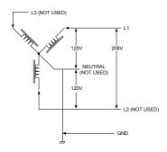
↑ Caution: The unused leg (L3 in the illustration) must remain open. Do not connect to a neutral bar, or to earth around.
