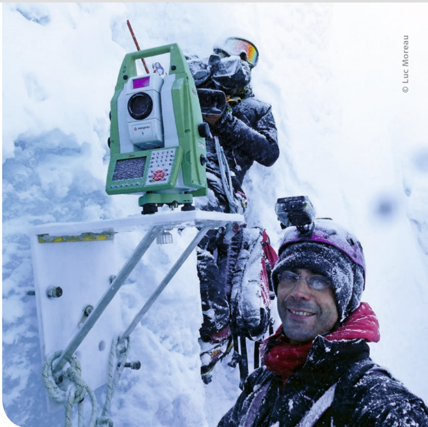
■ A bracket on the ice wall carries the MS50 to scan the moulin.
