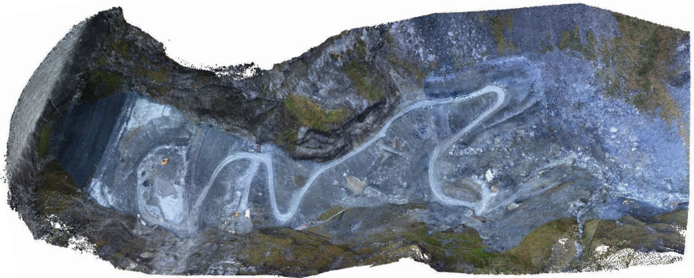
■ Generated point cloud of the area with an accuracy of up to one centimetre (0.4 inch).
