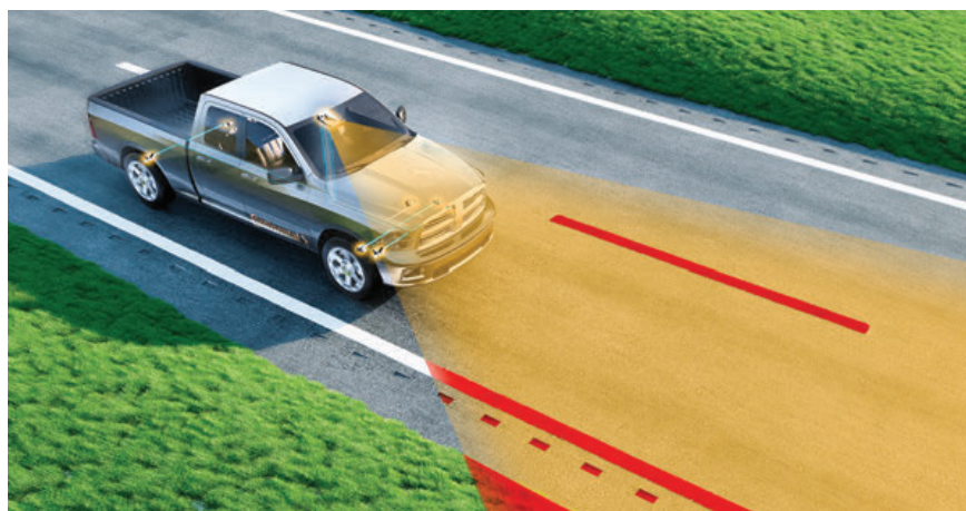
Continental's Road Departure Protection sensor detects the vehicle's lane position.
