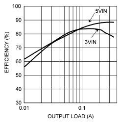
Figure 3. LM2735X  $\eta$  vs Load Current,  $V_{o}$  = 12V
