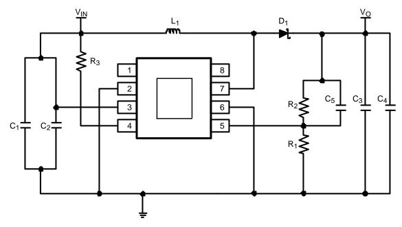
Figure 1. LM2735X 8-Pin MSOP-PowerPAD Schematic
