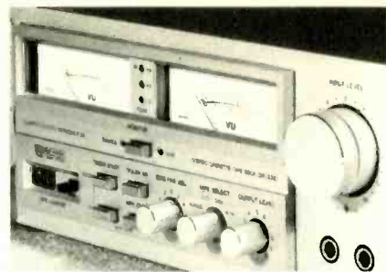
The Denon has both mechanical averaging meters and a set of fast, peak-reading LEDs for monitoring recording levels.
