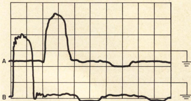
Fig. 10 Line with parallel loads. A is voltage waveform at t_d = 2.0 usec and B is voltage waveform at t_d = 0 usec.
