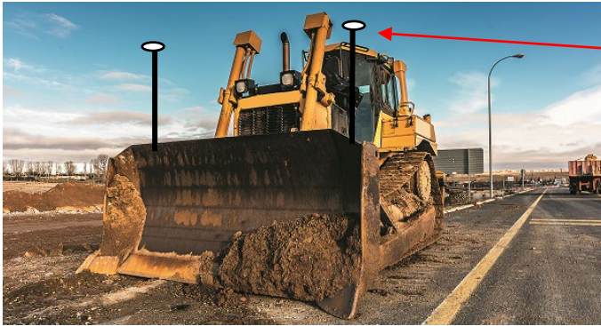
Figure 15: Antenna placement in heavy machinery/machine control application
