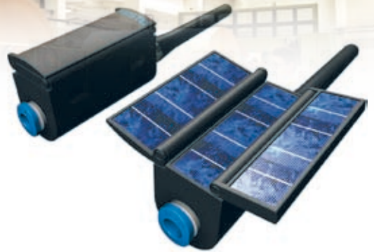
Right: Design study for energy-autonomous compressed-air sensor with EnOcean technology. Demonstrator from festo.
