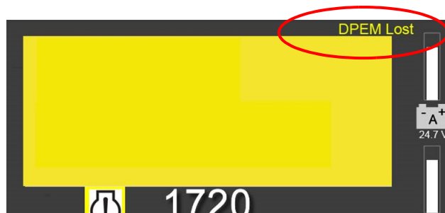
Figure 2-16 DPEM lost fault screen (sample)
