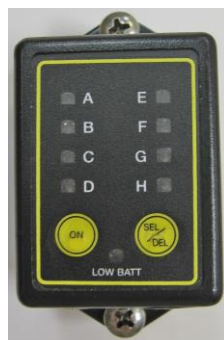
Figure 172. Data Logger Front View
