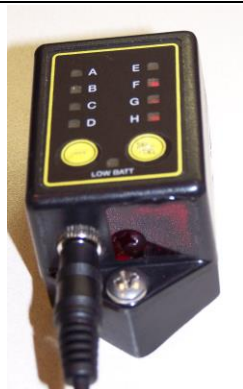
Figure 168. IR Bottom Of Data Logger
