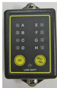
Figure 176. Data Logger Front View
