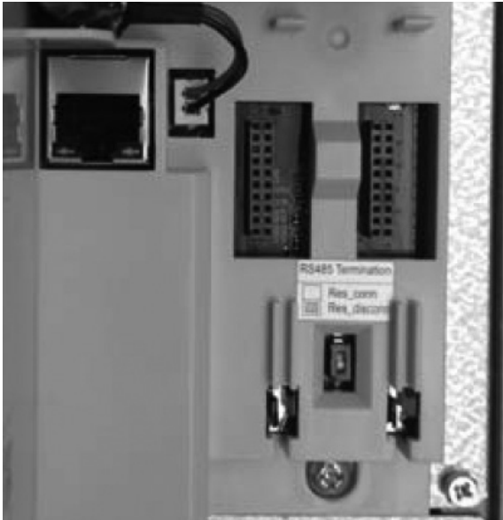
Figure 33. RS-485 Bus termination setup
