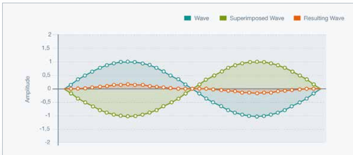
Figure 8: Negatively superimposed wave, destructive interference
