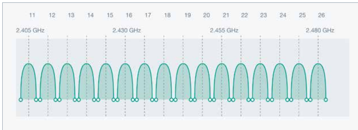
Figure 26: Channel designation in 2.4GHz band according to IEEE 802.15.4
