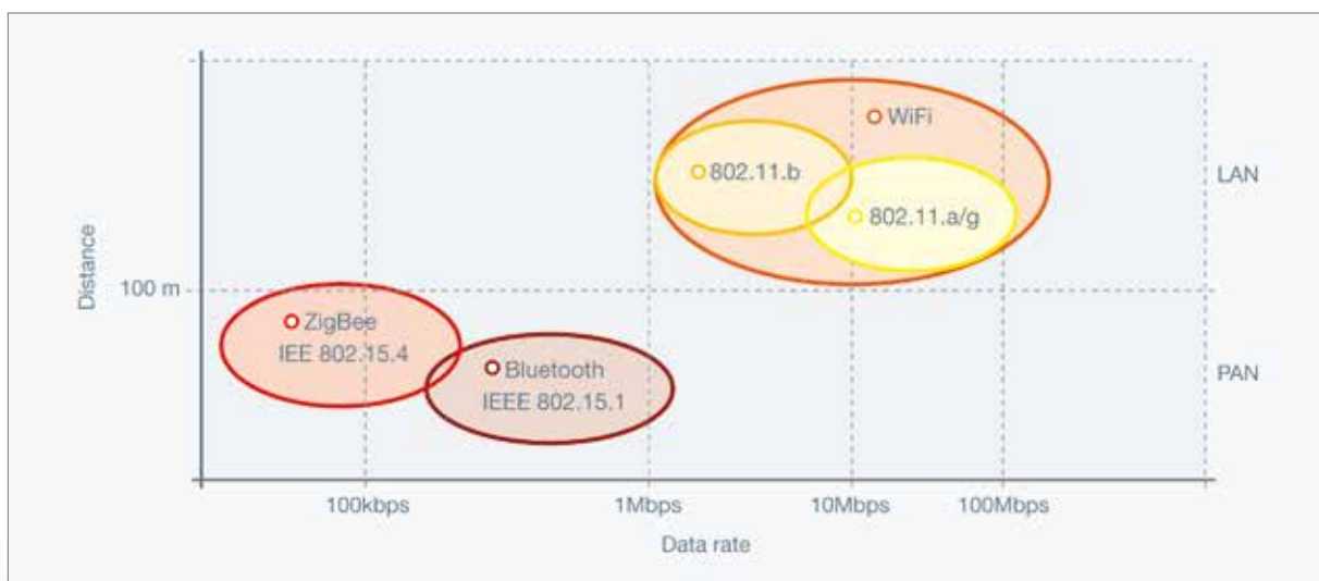
Figure 28: Wireless standards and their properties with respect to range and data rate
