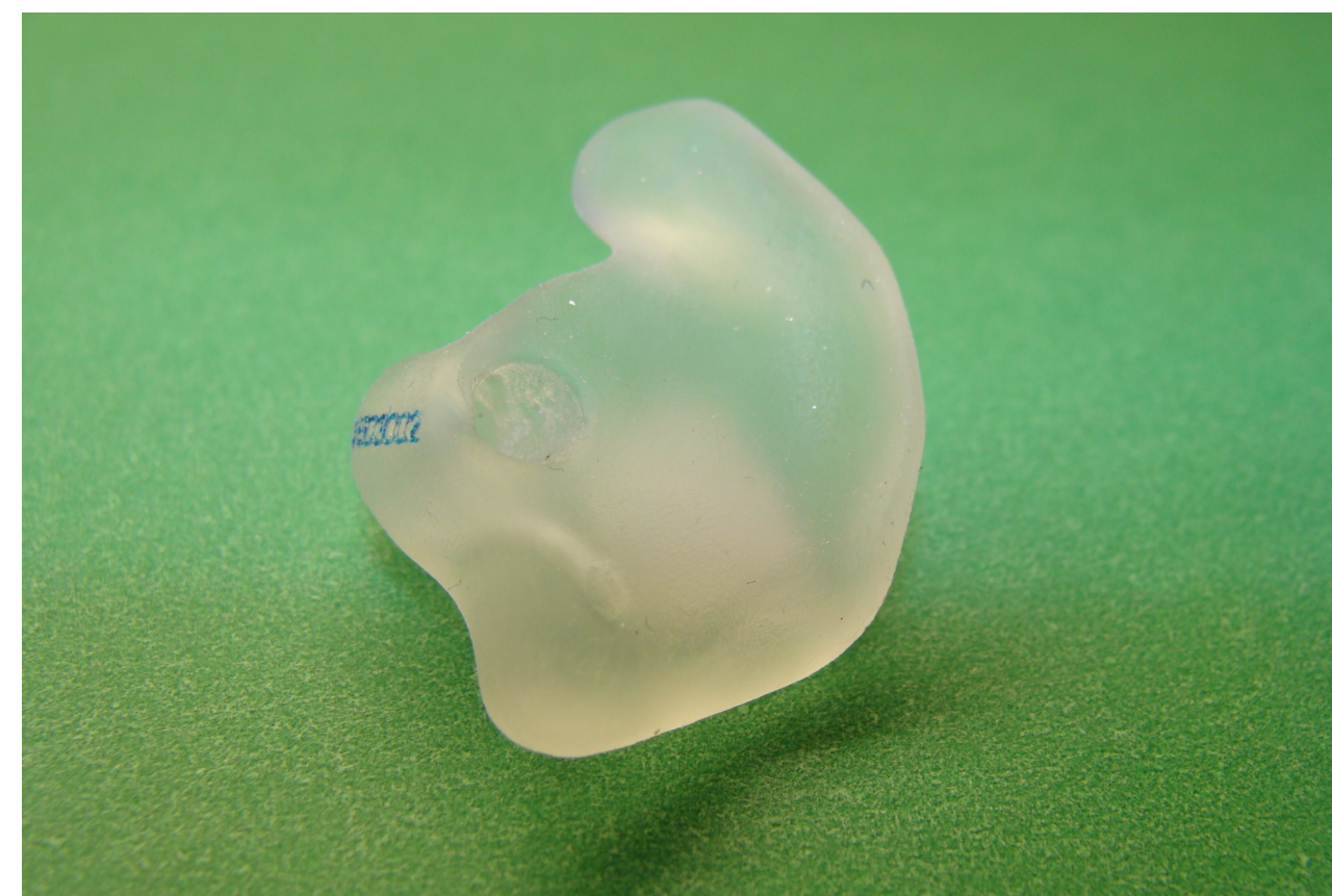
Figure 4. A custom occluding earmold was made for each participant's left ear. A custom hole was drilled into the earmold to allow the probe tube to be routed through without introducing additional acoustic leakage around the earmold seal within the ear canal.
