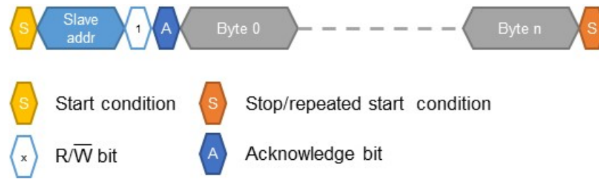
Figure 6. I2C Read operation description
