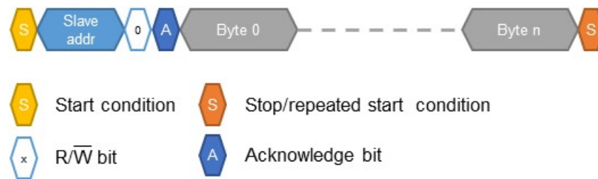
Figure 7. I2C Write operation description
