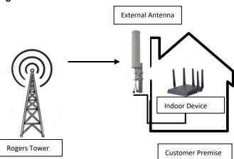
Diagram 1 – LTE Fixed Wireless Access Network Architecture
