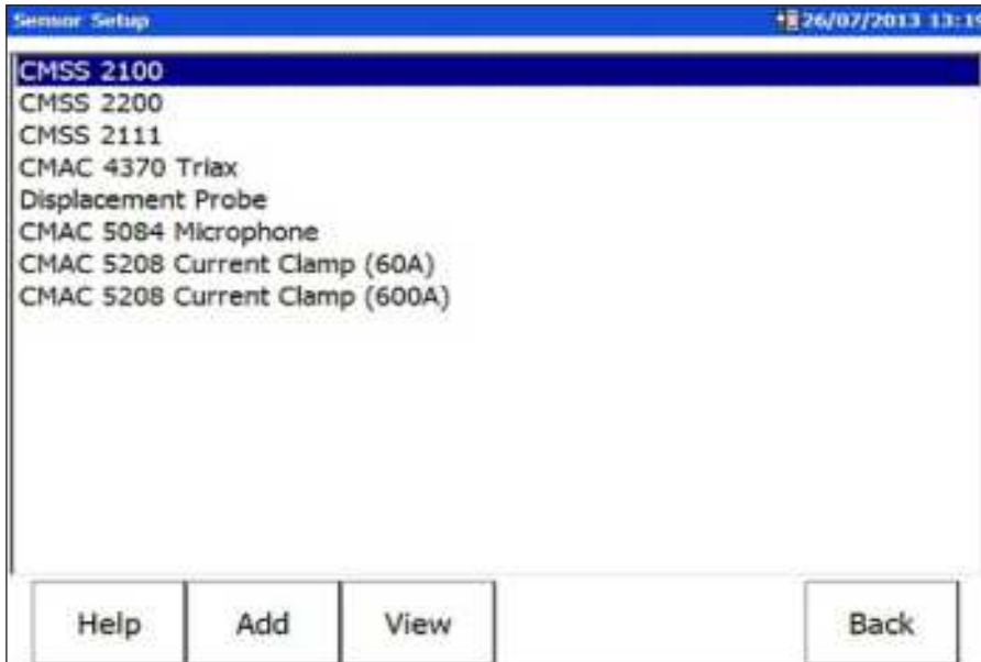
The SKF Microlog AX series Sensor Setup screen showing default sensors.
