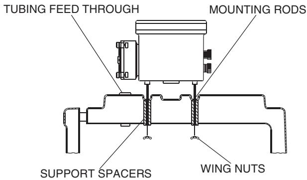
Figure 6-7 Mounting the Control Box
