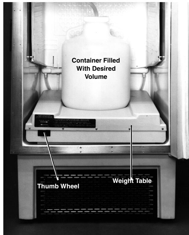
Figure 2-6 Sampler Shut-off Calibration
