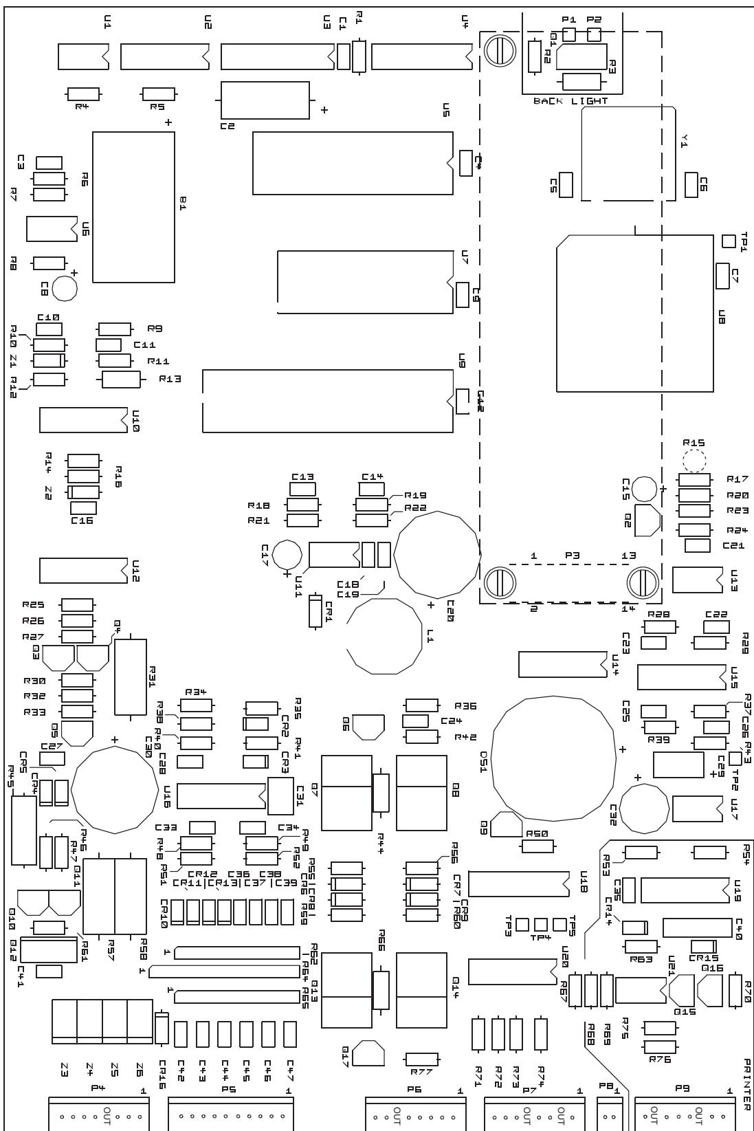
Figure 6-11 3710 Main Circuit Board Component Layout
