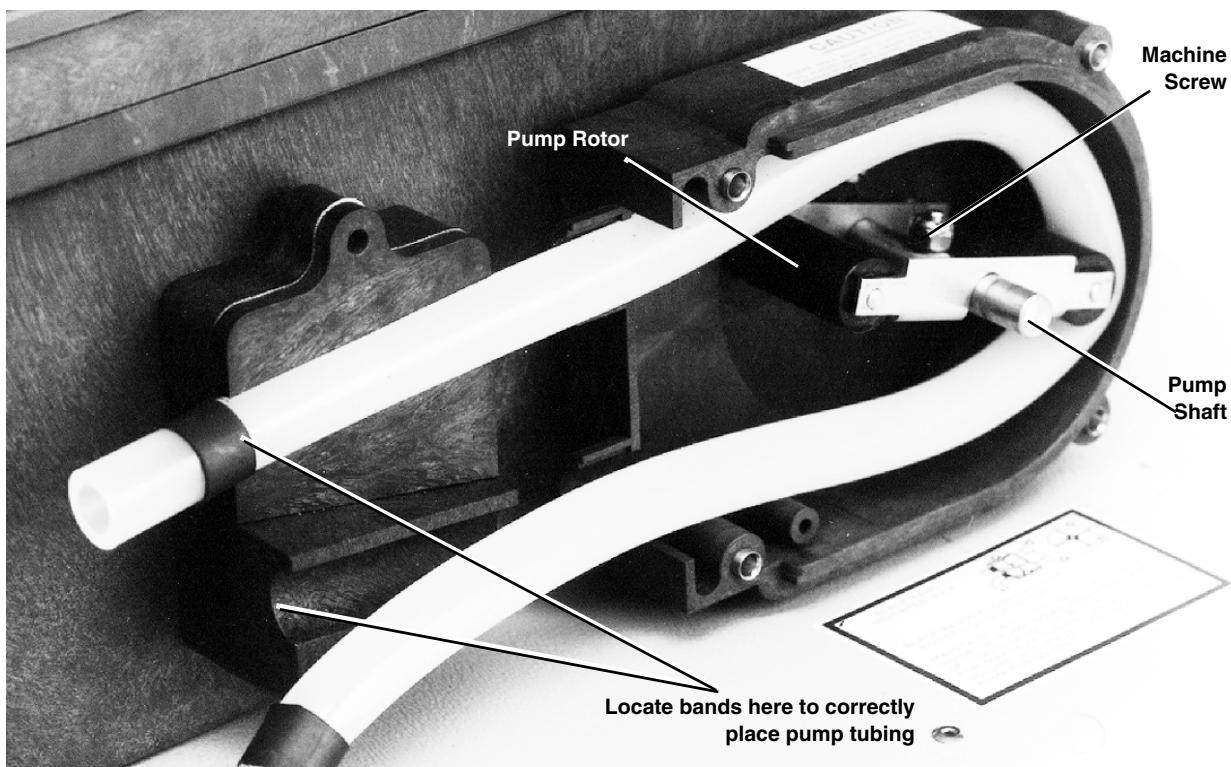
Figure 5-2 Pump Tube and Interior of Liquid Detector
