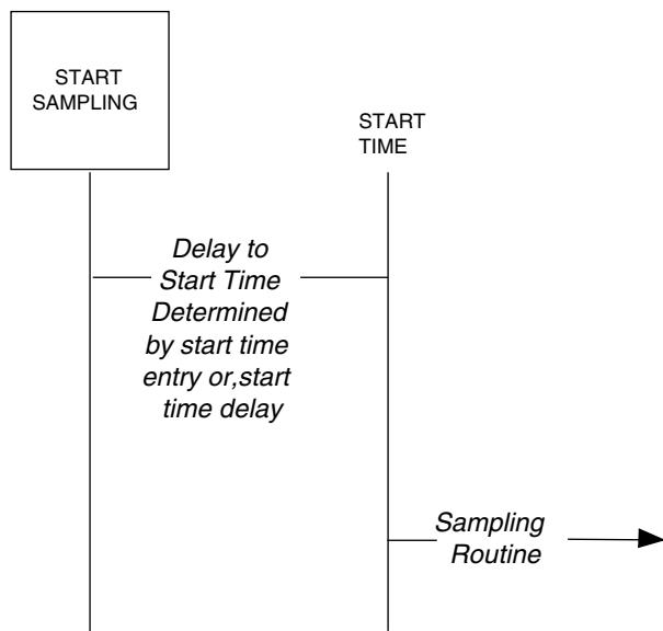
Figure 3-6 Simplified Start Time Diagram
