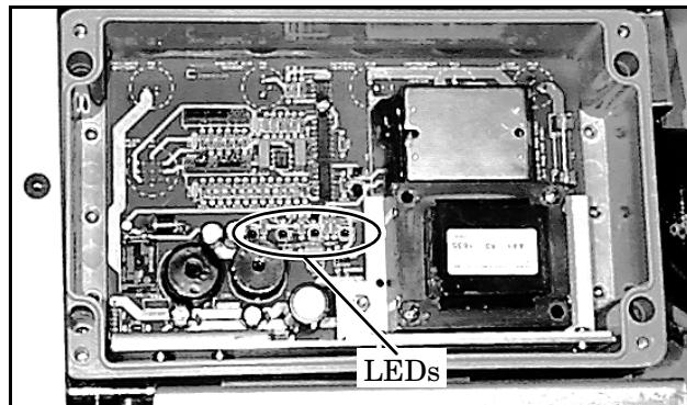
Figure 6-2 Thermostat Logic Circuit Board
