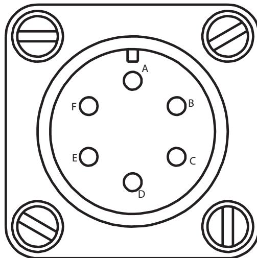
Figure 4-1 6-pin Connector Diagram
