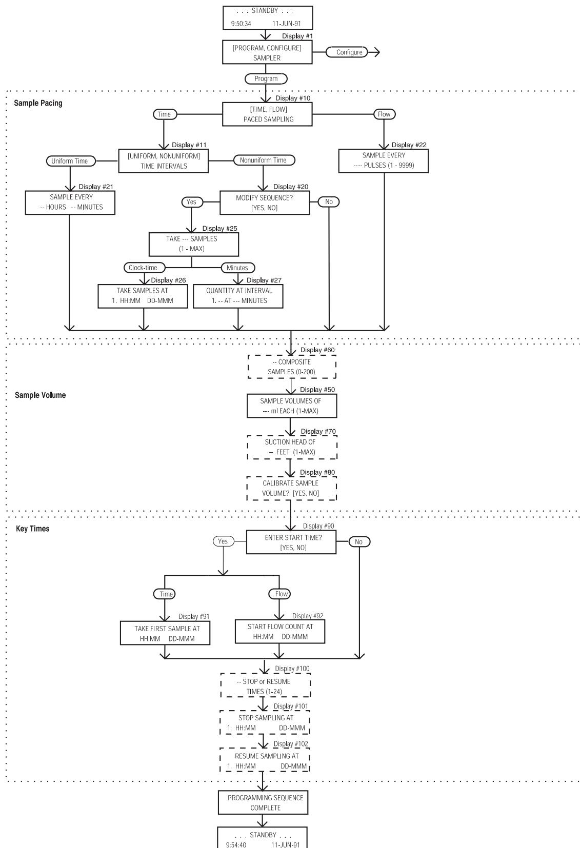
Figure 3-5 Extended Programming Mode: Program Sequence Structure
