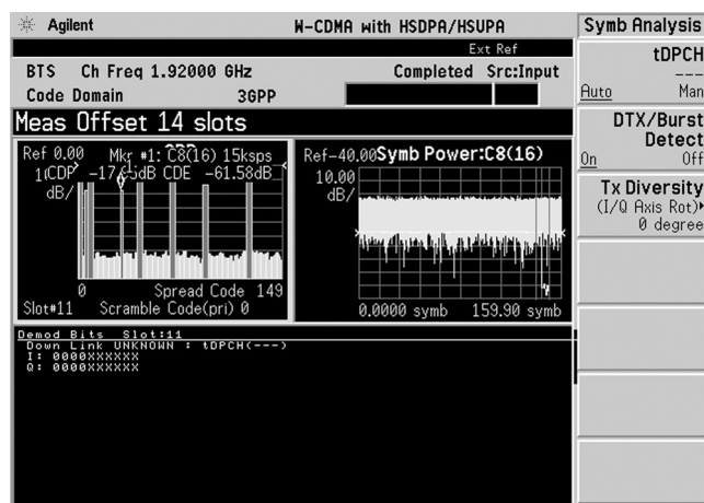
Figure 8. Symbol power and demodulated I/Q bits
