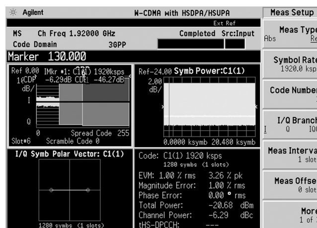
Figure 13. Symbol analysis of E-DPDCH in spreading factor 2 (1920 ksps)
