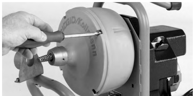
Figure 16 – Loosen 4 Drum Screws About 3 Full Turns But Do Not Remove
