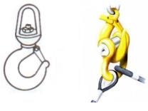
Hook with safety latch Correct positioning of shackle
