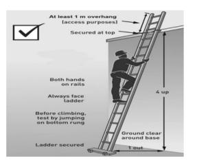
Figure 12: Correct set-up of ladder
