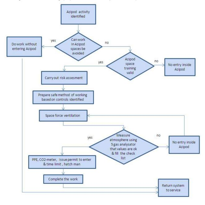
Flow diagram for use in drawing up a permit to enter the Azipod confined space:
