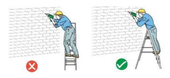
Figure 14: Correct use of step ladders
