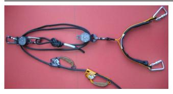
Figure 29: Example of pre-assembled lifting equipment, ready to use in emergency
