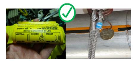
• In the case of lifting equipment that can be used in different configurations, the information of the working load limit must be kept with the lifting equipment.
