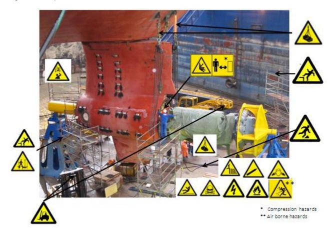
Figure 33: Typical risks when overhauling a shaft line at a dry dock
