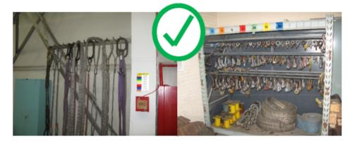
Figure 34: Storage of lifting accessories
