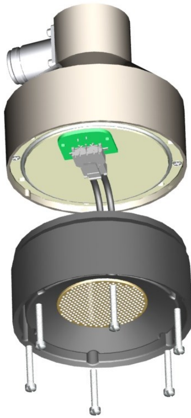
FIGURE 9-3. Remove transducer housing and disconnect wires
