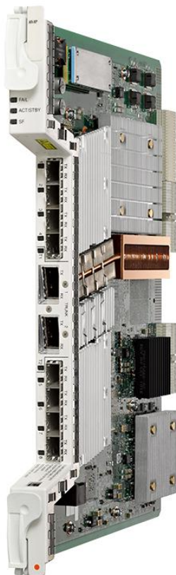
Figure 1. Cisco ONS 15454 Any Rate Enhanced XPonder Card
