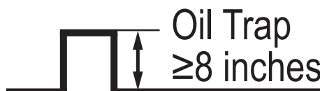
Figure 42: Close Up of An Inverted Oil Trap.
