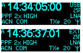
If powered from USB, USB is displayed in the upper right corner of the display instead of the battery symbol.
