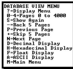
All data contained in the module's database is available for viewing using the commands. Refer to Modbus Protocol Specification (page 127) for information on the structure of Modbus messages. Each option available on the menu is discussed in the following topics.
