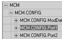
**Note:** Any changes made within either the MCM.CONFIG array must be downloaded to the MVI56MCM module by setting either the WarmBoot, ColdBoot, or cycling power to the module.
