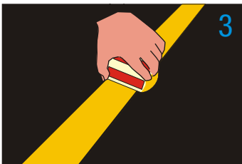
The RPM is fixed firmly by driving in the shanks
