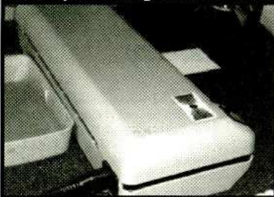
A 2" x 3" circuit board is inserted into the front of the SuperFuser. A few minutes later it comes out the back and drops into a water tray.
