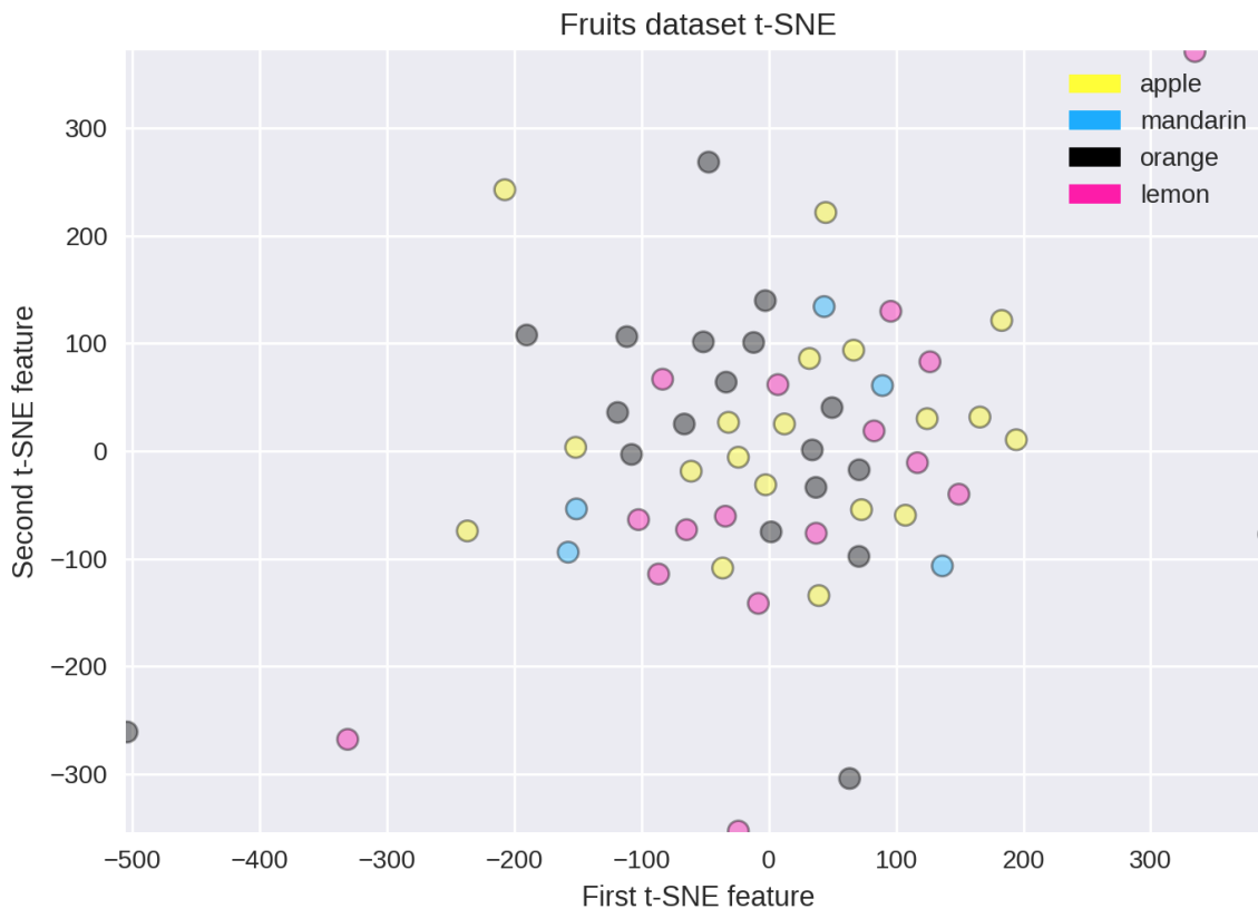
Fig. 2: You can see how some dimensionality reduction methods may be less successful on some datasets. Here, it doesn't work as well at finding structure in the small fruits dataset, compared to other methods like MDS.
