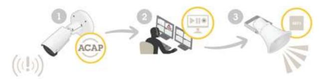
This example explains how to set up the audio device so that an action button appears when motion is detected. The action button can be used by the operator to play an audio clip.
