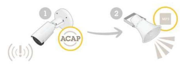
This example explains how to set up the audio device to play an audio clip when an Axis network camera detects motion.
