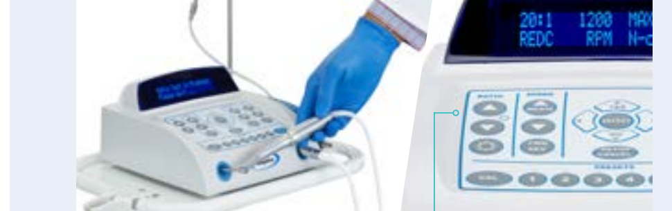
Aseptico's dynamometer calibration system allows dentists to diagnose the health of a handpiece.
