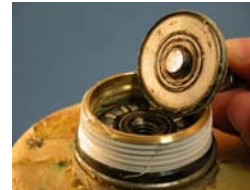
Unscrew Bolt, Remove Thrust Washer
