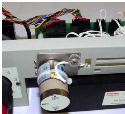
Figure B-25. Low-Pressure Valve Installation (Left Valve Mounting Position)
