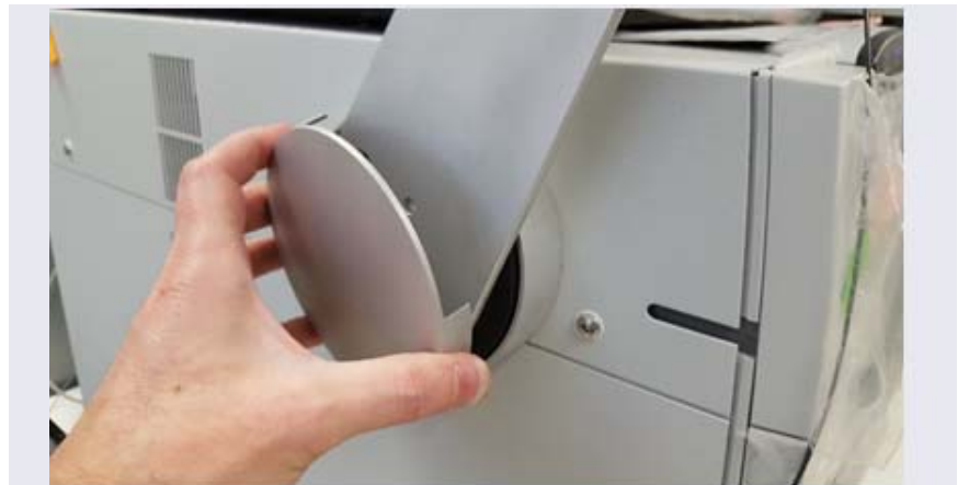
Figure 3-31. Reattaching the Cover of the Tablet Mounting Arm/Holder
