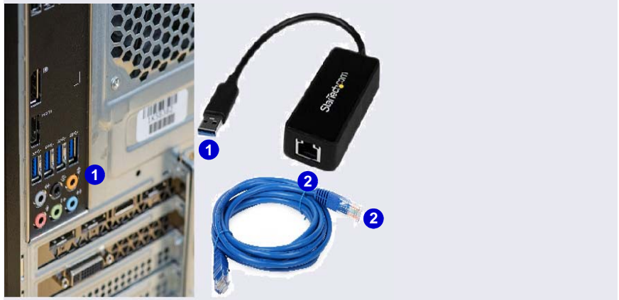
Figure 3-42. Ethernet USB-to-LAN Connection
