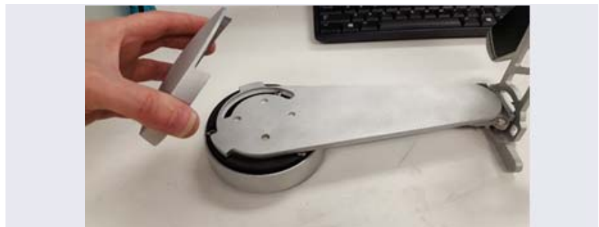
Figure 3-27. Removal of the Mounting Arm Cover
