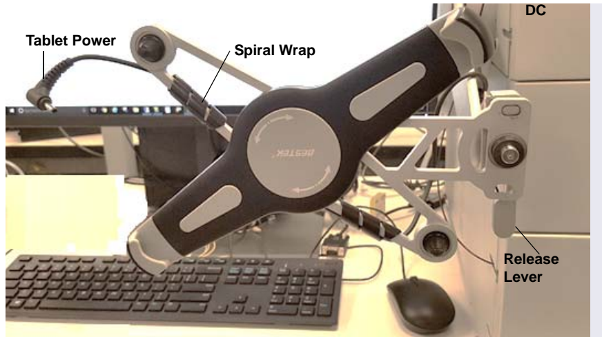
Figure 3-37. Tablet Connections and Viewing Adjustment
