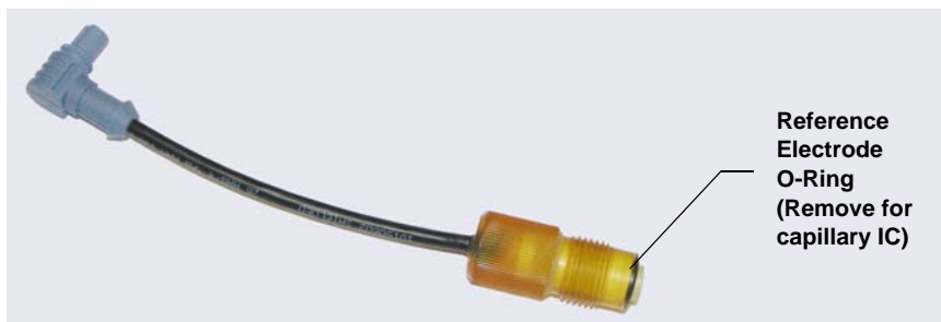
Figure B-8. pH-Ag/AgCl Reference Electrode O-Ring
