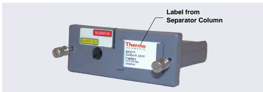
Figure 4-9. Capillary Column Tray with Column Label
