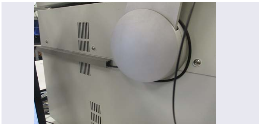
Figure 3-35. Tablet Wiring Duct Attached to the DC
