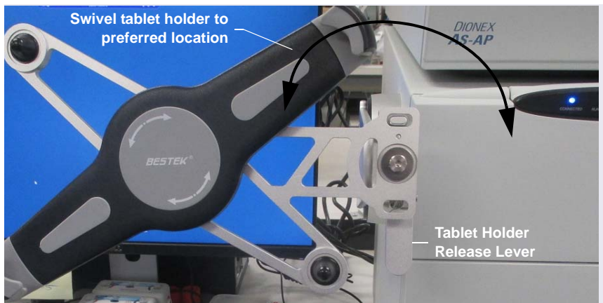
Figure 3-36. Tablet Connection and Viewing Adjustment
