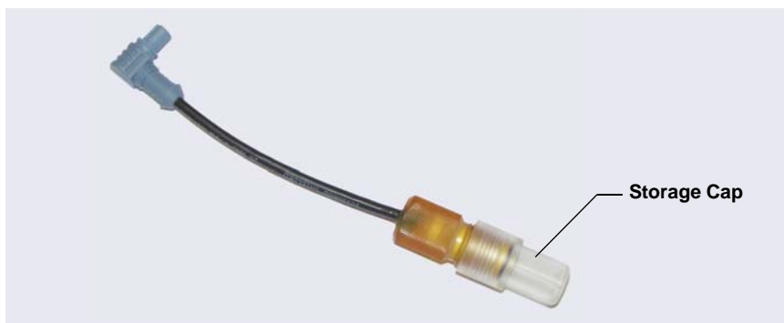
Figure B-7. pH-Ag/AgCl Reference Electrode in Storage Cap
