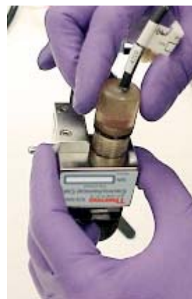
Figure B-11. Installing the pH-Ag/AgCl Reference Electrode In the Reference Electrode Well
