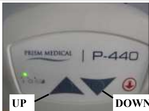
Figure 5C - Hand control showing raising/lowering buttons
