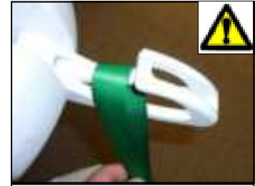
Figure 3 - Sling loop incorrectly resting on the P-440 hook locking clip.
