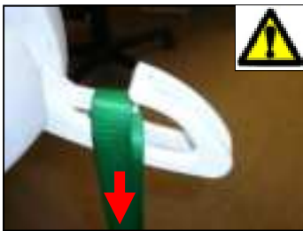
Figure 4 - Load applied to the P-440 locking clip. The sling loop begins to slide off the hook locking clip.
