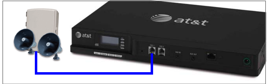
Figure 10. Single-Zone Overhead Paging on FXS Port
