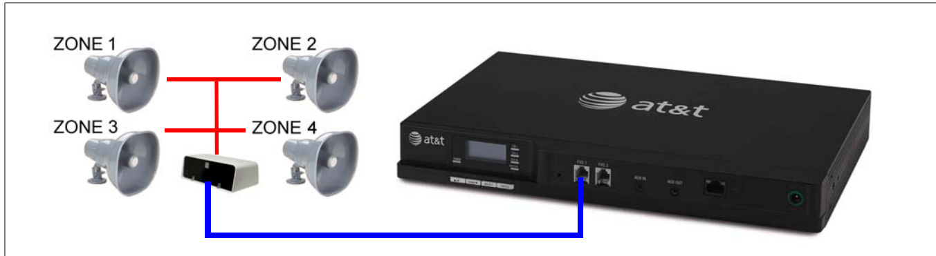
Figure 11. Multiple-Zone Overhead Paging on FXS Port
