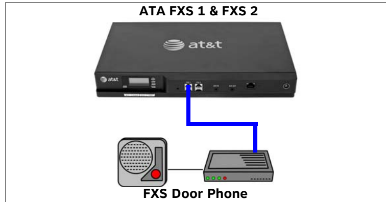
Figure 12. Station Port (FXS) Door Phone Connection
