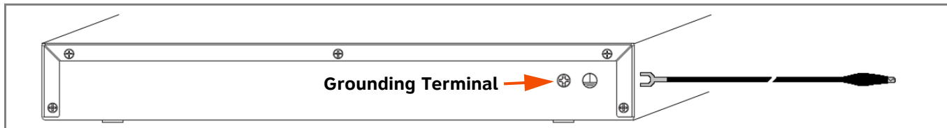
Figure 19. T1 Gateway and ATA Grounding
