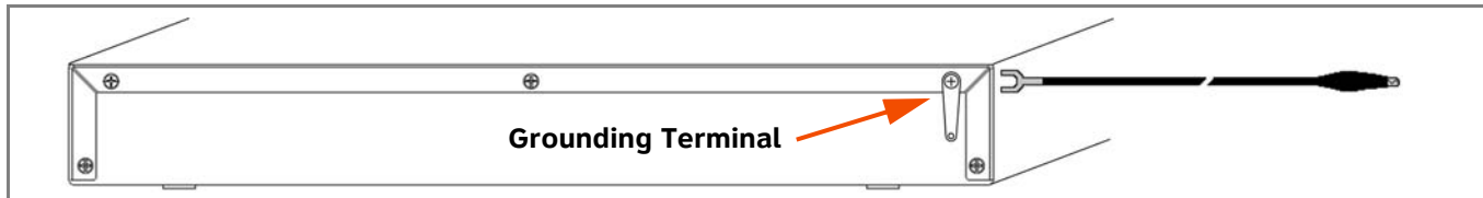
Figure 18. PSTN Gateway Grounding
