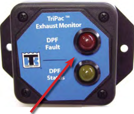
Red DPF Fault Indicator Light on Exhaust Monitor
