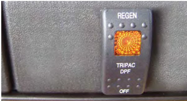
Amber Indicator Light on Regeneration Switch
