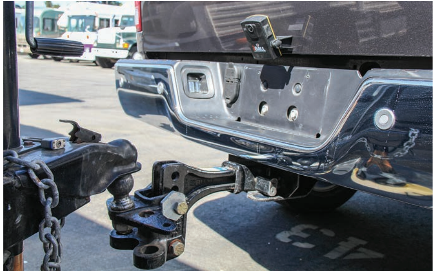
The iBall can be used on any vehicle with a steel skin and can be easily positioned for the best view of the ball mount and trailer coupler. (License plate removed for photos.)
