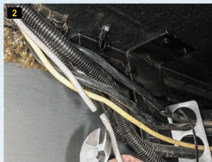
1) The dome was mounted close to the air conditioner, which was contrary to the installation instructions. At this point, the roofline is not level, exceeding the limit suggested in the instructions. However, the antenna performed better than expected in this location. 2) After discovering a kink and slice in the factory coax that prevented the Quest from operating, the cable was cut to make way for better-quality RG-6 coax. 3) To repair the factory coax, the wire was stripped using a tool acquired at a home-improvement store.
