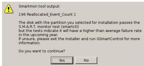
Figure 2-17: SMART warning of risk of failure
