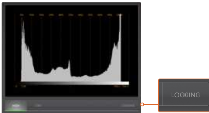
From the Histogram Display, select the Logging button to switch to the Error Logging Display.
