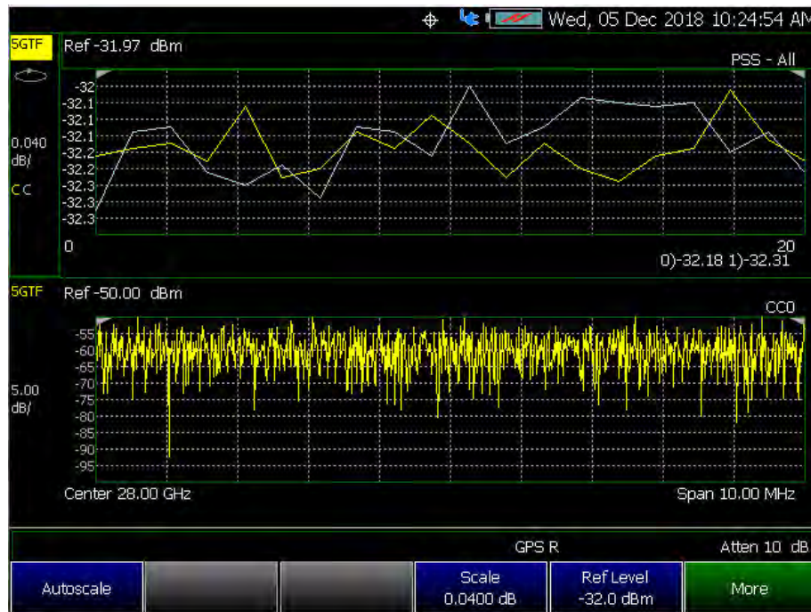
Figure 12-21 Spectrum and Strip Chart Display Type – 5G TF
