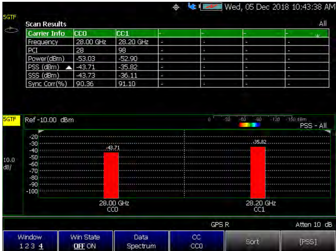
Figure 12-10 Example of 5G TF Single Carrier and Single Cell
