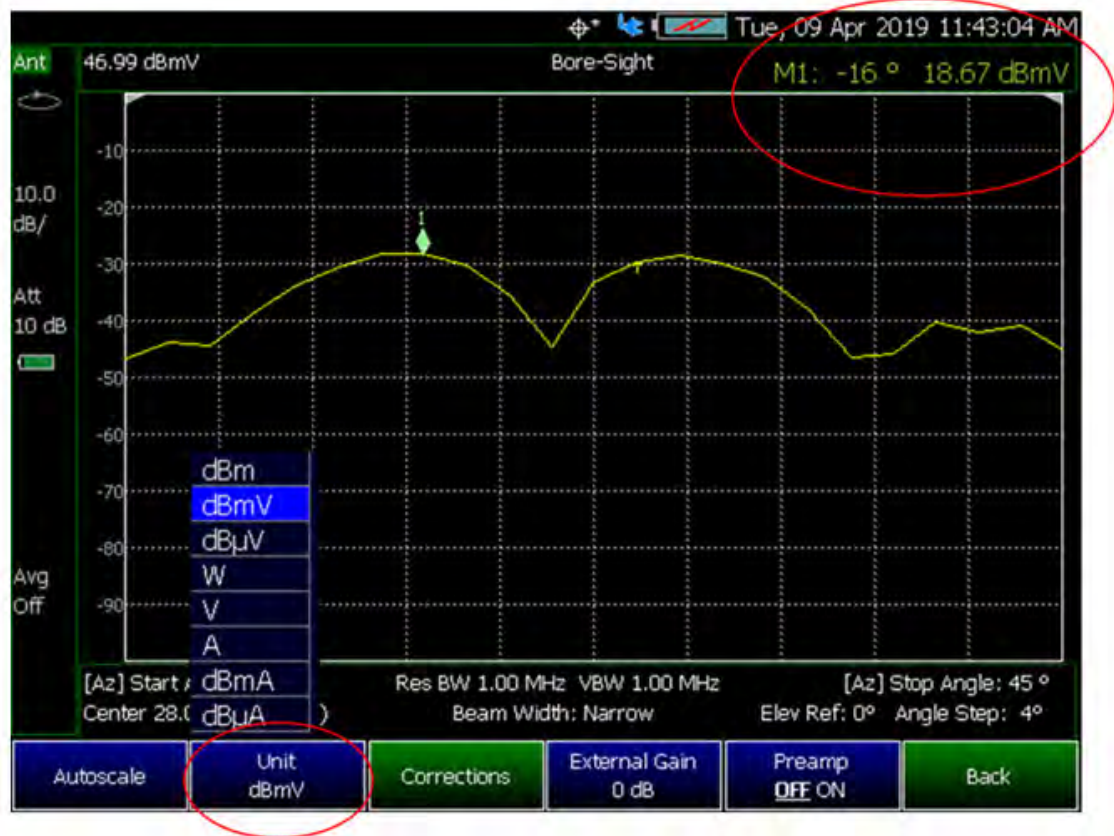
Figure 15-22 Field Strength Annotation that can be Recorded and Played Back
