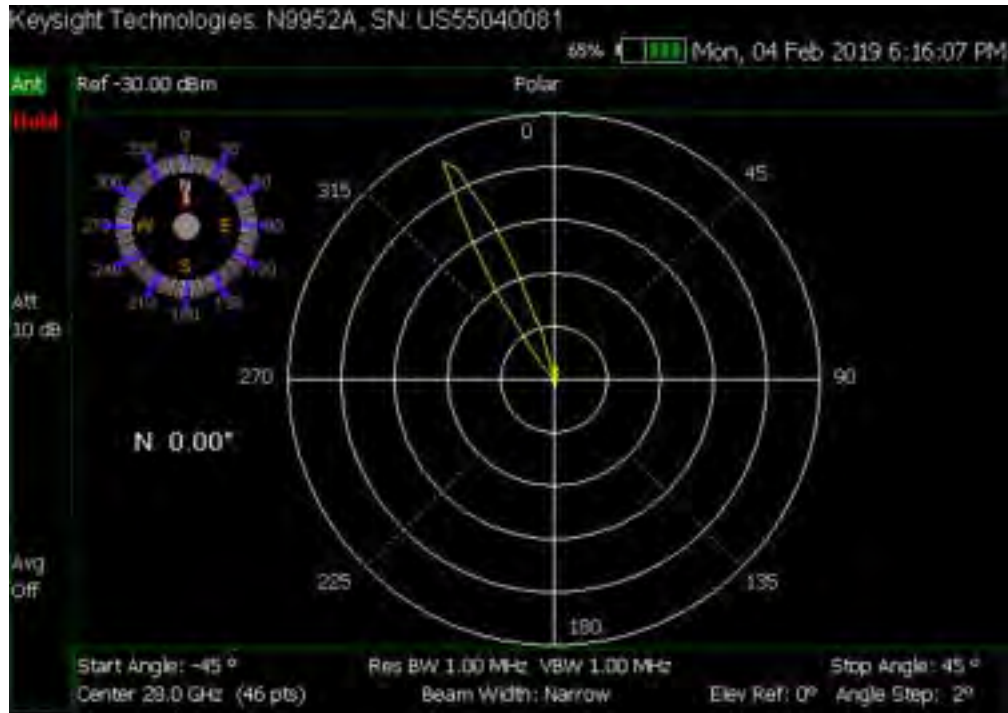
Figure 13-3 Polar Scan with compass displayed
