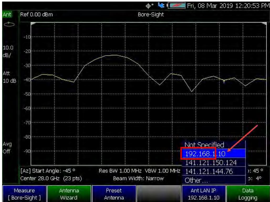
Figure 13-15 Example of Phased Array Antenna and FieldFox Static IP Setup - First Three Static IP Fields Are the Same
