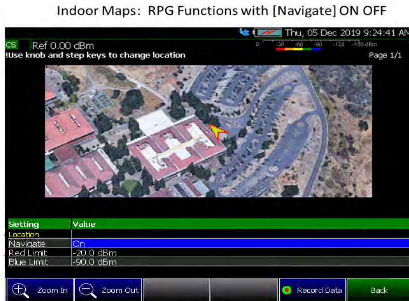
Figure 15-3 Using Mapping (Option 352) - Satellite View for Indoor Mapping
