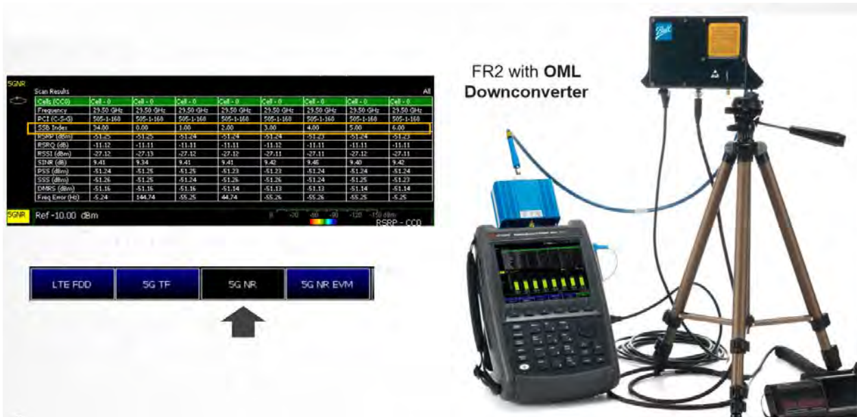
Figure 12-11 Example of 5G NR Single Carrier and Single Cell
