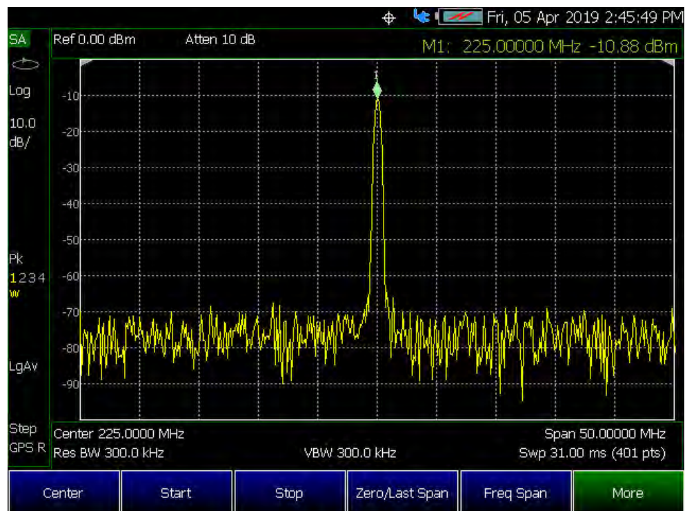
IF Output Wide with CF=225 MHz (Requires Option B04 or Option B10)
