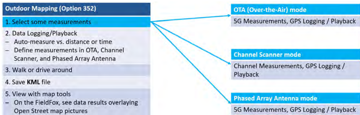
Figure 15-13 Overview – Setting Up Option 352 (Outdoor Mapping) Using Other Modes
