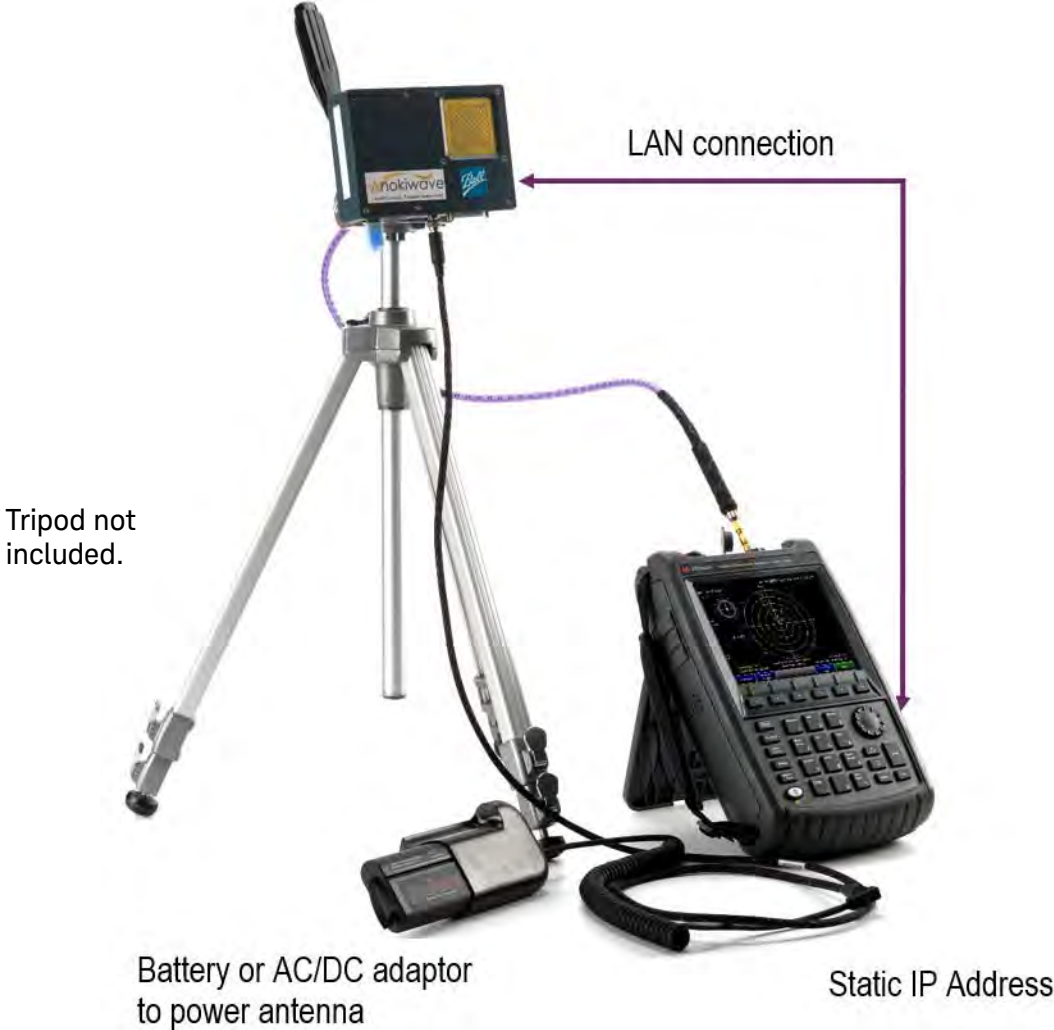
Figure 13-1 Example of local point-to-point LAN connection
