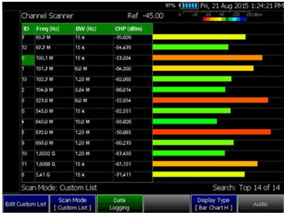
Figure 26-6 Bar Chart Horizontal Display Type
