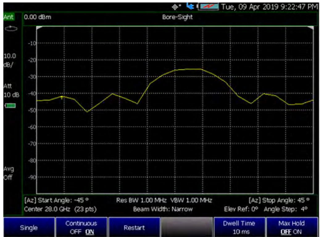
Bore-Site Measurement with CW RF (Dwell Time=10 ms, Max Hold=OFF)
