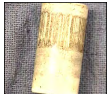
Figure 5-8. Examine Ceramic Plungers
