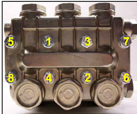
Figure 5-17. Torque Sequence in “X” Pattern
