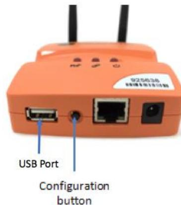
**Note** If you proceed to Step 5 before the self-test sequence ends, the bridge enters configuration mode rather than upgrade mode.
