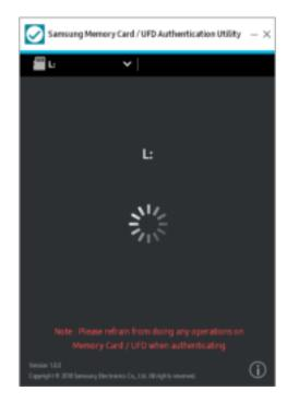
3. If there is no Memory Card/UFD connected to PC, Utility shows "Insert a Memory card / USB Flash Drive" message. Then, if user inserts a Memory Card/UFD, Utility automatically recognizes and authenticates it.
