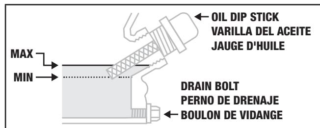
5. Add oil according to "Add Engine Oil" on Assembly section. DO NOT OVERFILL. Oil not included for routine maintenance.
