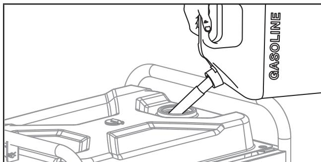
5. Screw on the gasoline cap and wipe away any spilled fuel.
