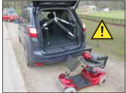
4. Keeping hold of the handset, move clear of the Smart Lifter and its path of operation.
