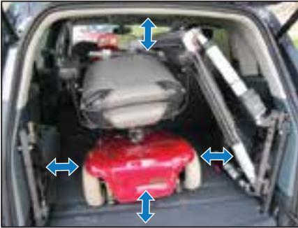
7. Ensure there is clearance for the Smart Lifter to swing fully outwards.
