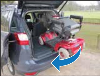
12. Press and hold the left or right button (depending on the side of installation) to move the scooter inwards. Rotate the scooter as it moves inwards.
