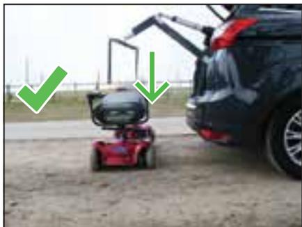
7. Position the scooter so that the lifting point is directly beneath the spreader bar. Ensure the scooter is folded/seat off.
