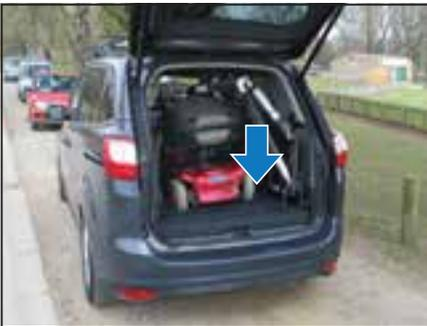
14. Press and hold the down button until the scooter is firmly placed onto the floor of the vehicle and the straps become loose enough to detach.\*
