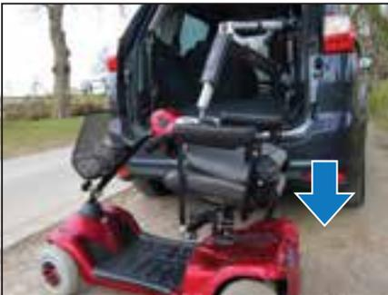
9. Press and hold the down button until the scooter/chair is grounded and there is some slack in the lifting straps.\*
