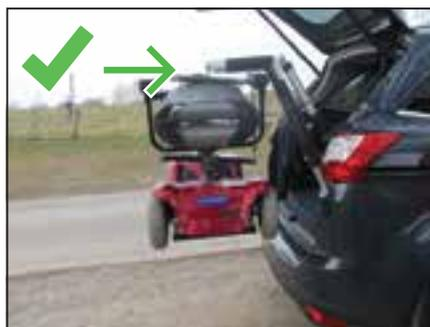
11. Release the up button once the scooter has reached the upmost position.
