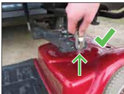
9. Engage the keyhole plates securely to the lifting bracket. (The bracket will vary depending on the scooter being lifted) DO NOT attempt to lift without all lifting straps securely connected.
