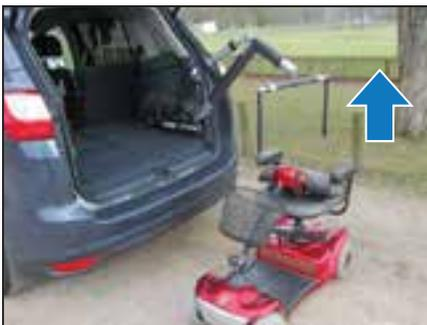
11. Ensure the scooter/chair is free from the Smart Lifter. Press the up button to raise the boom fully upwards.
