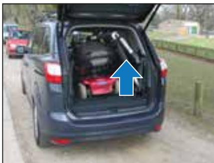
6. Press and hold the up button to raise the scooter/chair from the vehicle floor.
