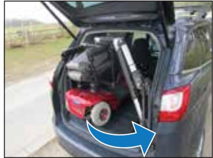
8. Press and hold the left or right button (depending on the side of installation) to swing the Smart Lifter outwards.
