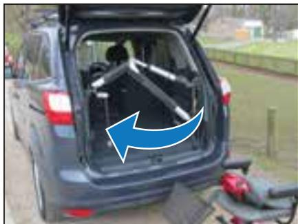
12. Press and hold the left or right button (depending on side of installation) to move the Smart Lifter inwards.\*
