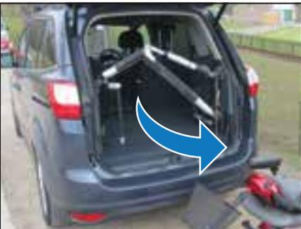
5. Press and hold the left or right button (depending on the side of installation) to swing the Smart Lifter outwards.
