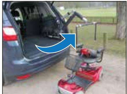
6. Release the button when the boom is at its outmost position.
