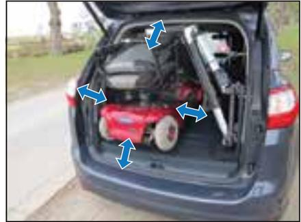
13. Guide the scooter into the boot, ensuring there is adequate clearance for the boom and scooter to swing into position.
