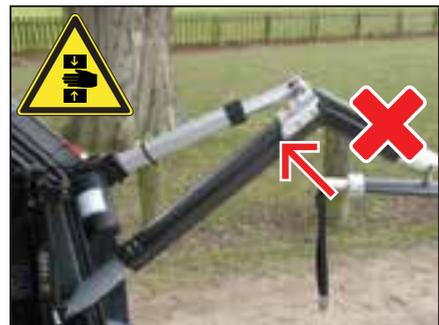
**WARNING!** - When lifting/lowering, do not hold or steady the Smart Lifter by placing your hand beneath the actuator. This is a pinch point and may cause injury.
