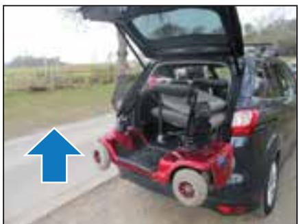
10. Press and hold the up button to raise the scooter from the ground.
