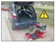
4. Keeping hold of the handset, move clear of the Smart Lifter and it's path of operation.
