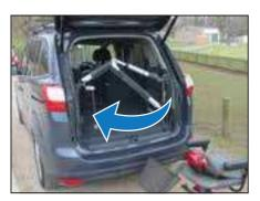
12. Press and hold the left or right button (depending on side of installation) to move the Smart Lifter inwards.\*
