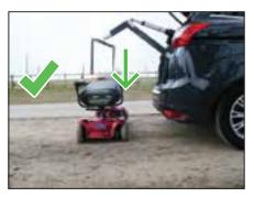
7. Position the scooter so that the lifting point is directly beneath the spreader bar. Ensure the scooter is folded/seat off.
