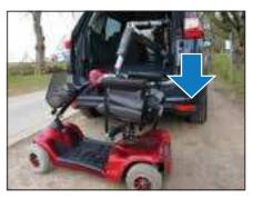
8. Press and hold the down button to lower the boom.
