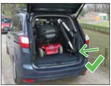
15. If fitted, you should engage the restraint system now.\*\*
