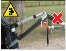
**WARNING!** - When lifting/lowering, do not hold or steady the Smart Lifter by placing your hand beneath the actuator. This is a pinch point and may cause injury.
