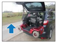
10. Press and hold the up button to raise the scooter from the ground.
