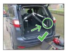
13. Return the handset to its stored position, ensuring the cable is clear of trapping points or hazards.
