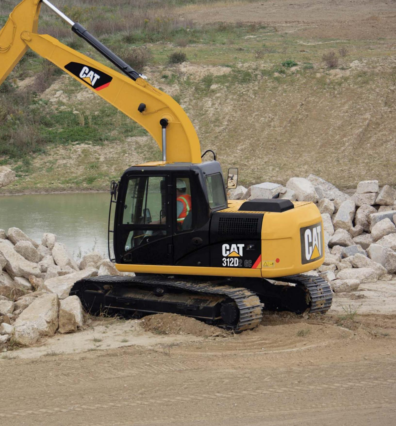
Good machine performance combined with low owning and operating costs make the Cat 312D GC Series 2 hydraulic excavator the preferred machine of choice for utility contractors. Unmatched versatility, improved controllability, easy operation, and a comfortable, redesigned operator station help make the 312D GC Series 2 an industry-leading performer.
