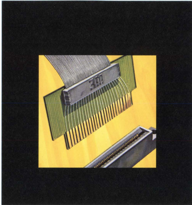
Printed Circuit Board Transitions. Transition flat cable to printed circuit boards simply and reliably. Up to 64 conductors on .050" centers can be terminated simultaneously with 3M's unique "U" contact principle.
