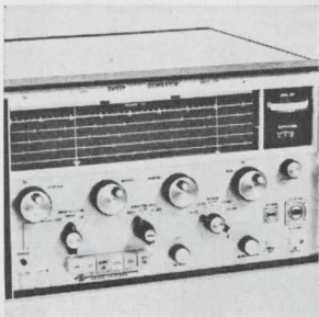
Sweep generator series 101 generates swept frequency signals from 0.1 to 24 Ghz without external plug-in units. Range is divided into 5 bands, selected by a front panel control: 0.1 to 4.2 Ghz, 4.2 to 8.2 Ghz, 8.2 to 12.4 Ghz, 12.4 to 16.4 Ghz and 16.4 to 24 Ghz. Continuous sweep is up to 4100 Mhz including 100 Mhz to 4200 Mhz range. Space Kom Inc., Box 10, Goleta, Calif. [401]
