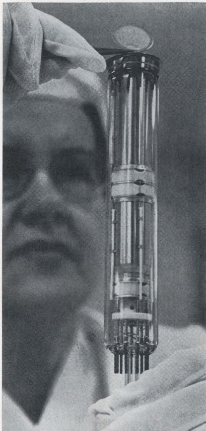
On target. A silicon-target vidicon is handled with care in one of its final assembly stages.
