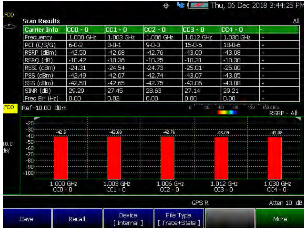
Figure 12-8 Example of LTE FDD with Multiple Carriers, Single Cell Site, and KPI's
