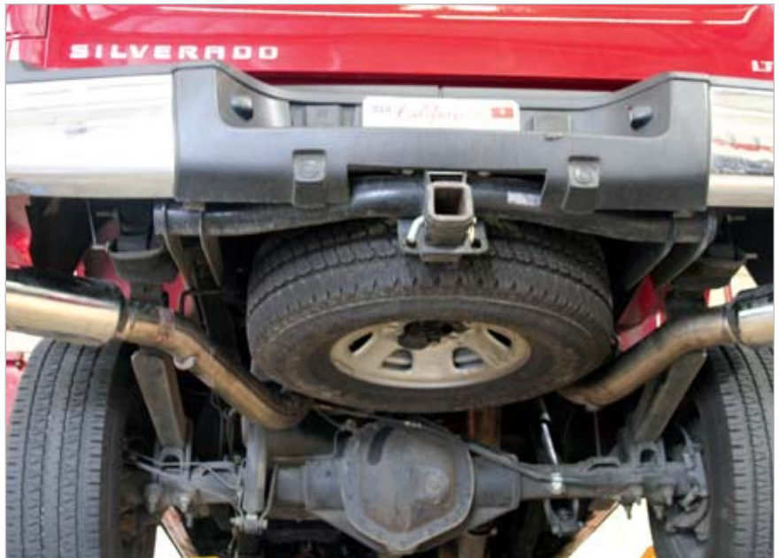
The Big Hoss kit we tried out had the optional dual exhaust, which splits just forward of the rear axle.
