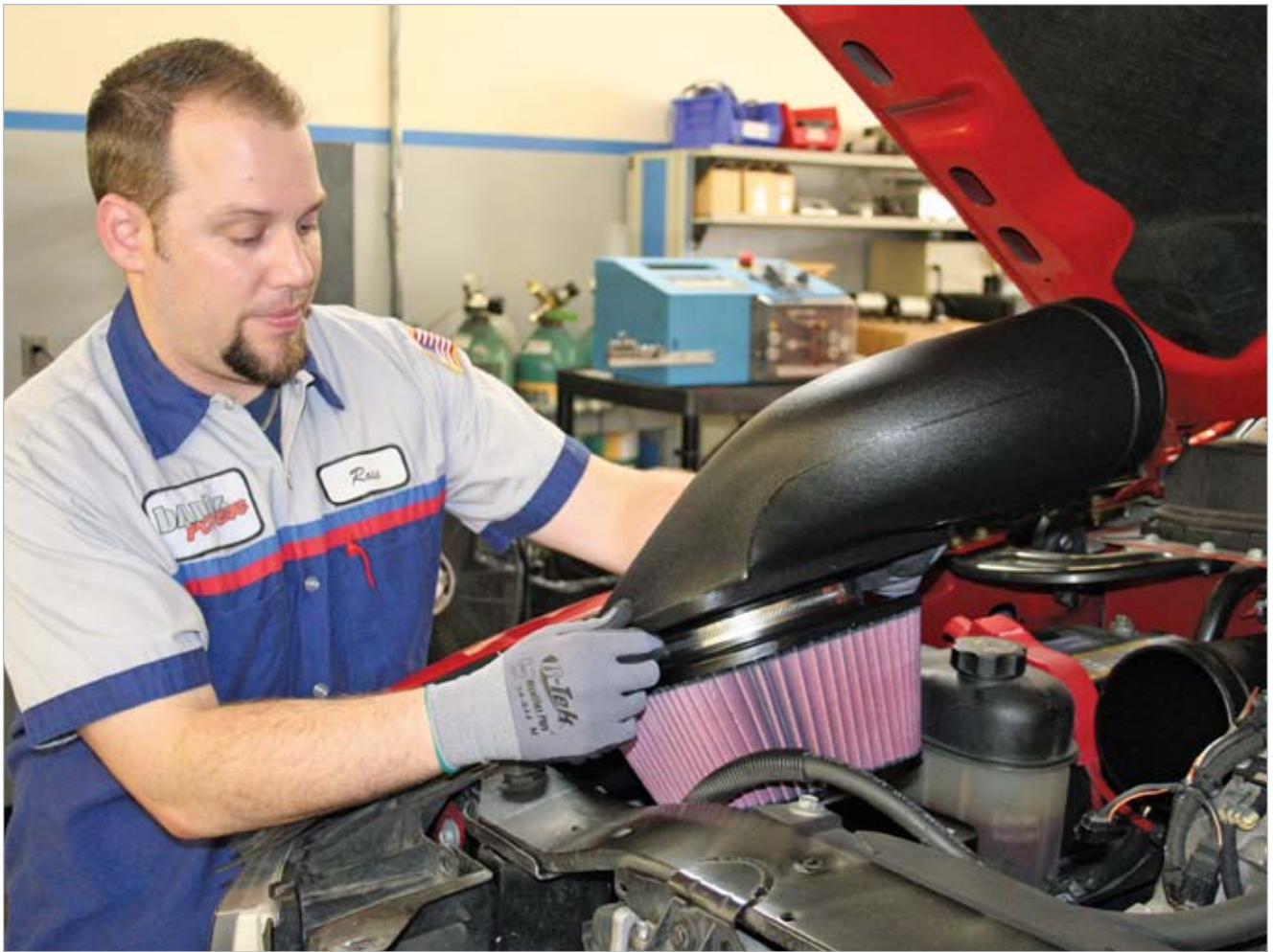
A Banks technician installs the Super Scoop intake with air filter.
