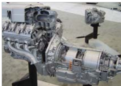
GM hybrid VVT V-8 engine with cutaway transmission
