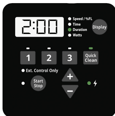
Figure 10: Setting Duration for Quick Clean
